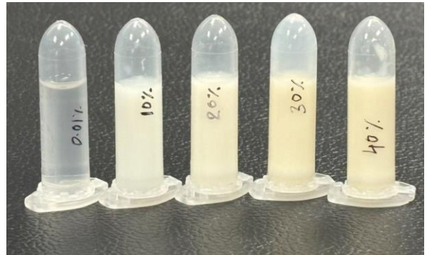
Fig.2: Silica nanoparticles dispersed in ethanol with varying weight percentages.
