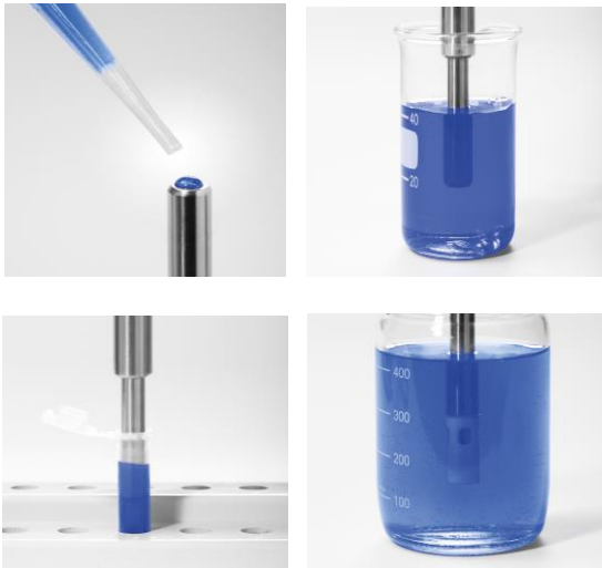
Fig.1: The dip-in probe of the NANOTRAC FLEX allows direct measurements in vessel: beaker, bottle, Eppendorf tube, or even a single drop of liquid.
