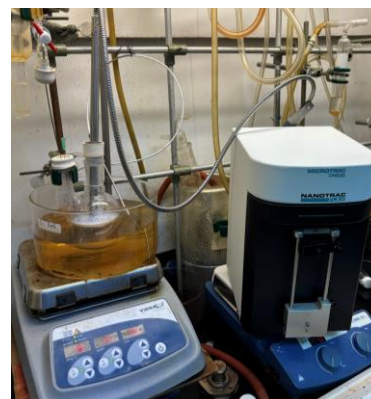
Fig. 1: Inserting Probe in Polymerization Reaction
