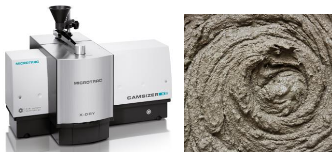
Figure 3: The CAMSIZER X2 is particularly suitable for mixed materials, containing fine powder and aggregates, like mortar or plaster.
