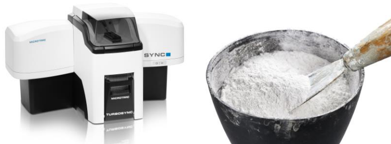
Figure 1: The SYNC analyzer with the TurboSYNC dispersion module is suitable for powdered bulk solids.
