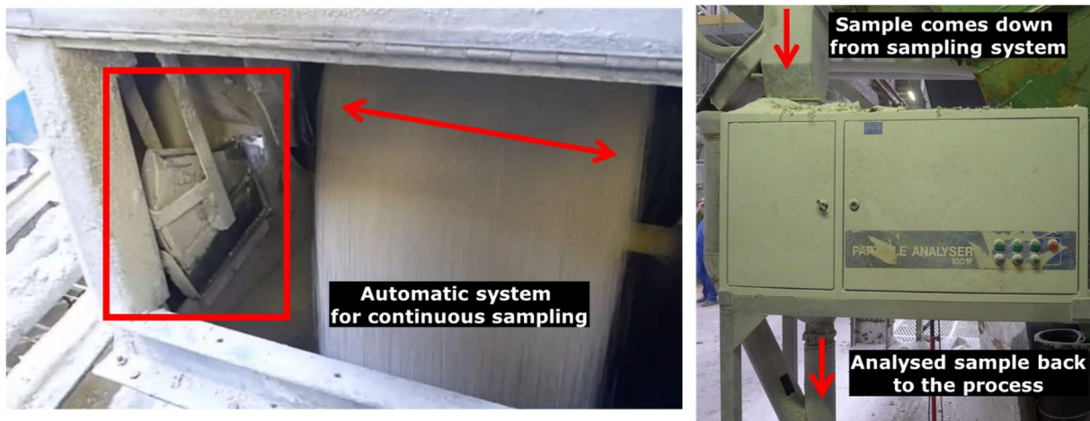
Figure 3: The sampler moves through the product stream from left to right and back. It takes approx. 0.5 - 0.8 kg sample at a time and transfers it to the image analyzer.
