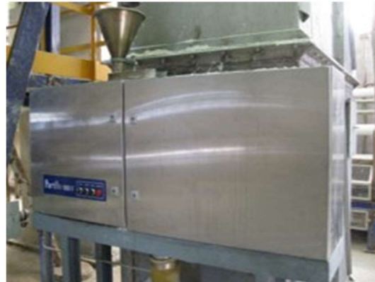
Figure 2: Left: On-line image analyzer in a fertilizer plant, working continuously since 1995 without service. Right: In-line image analyzer installed in December 2011
